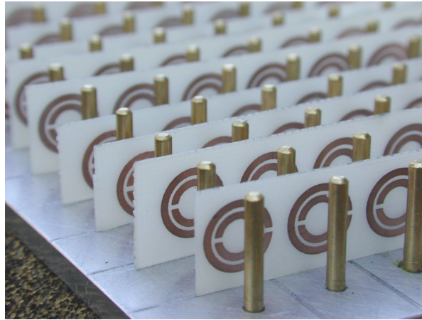
Figure 1.11 First composite structure of wire array and SRR array [43]
